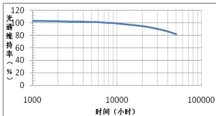
Remarks: This chart shows the actual testing data of many streets that exactly reflects luminous flux degradation of LED High bay lights in use. It is noticeable that natural environment conditions such as weather, temperature and so
